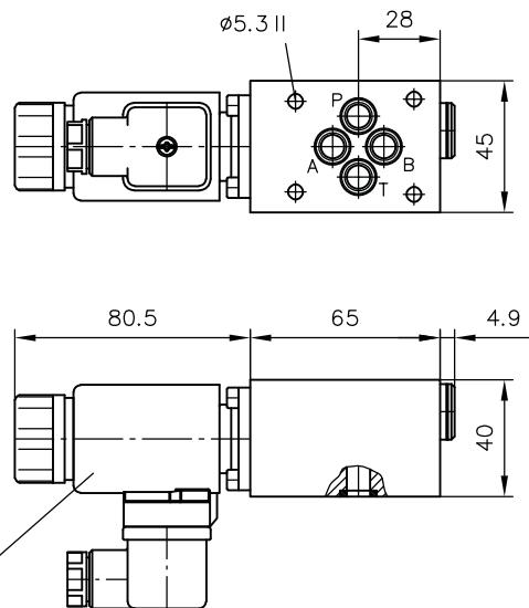
1 Solenoid GM..., WGM..., XM..., for other solenoid versions, see Chapter 4.5, "Intermediate plate with switchable pressure reducing valve at P: NZP 16 LZY"
