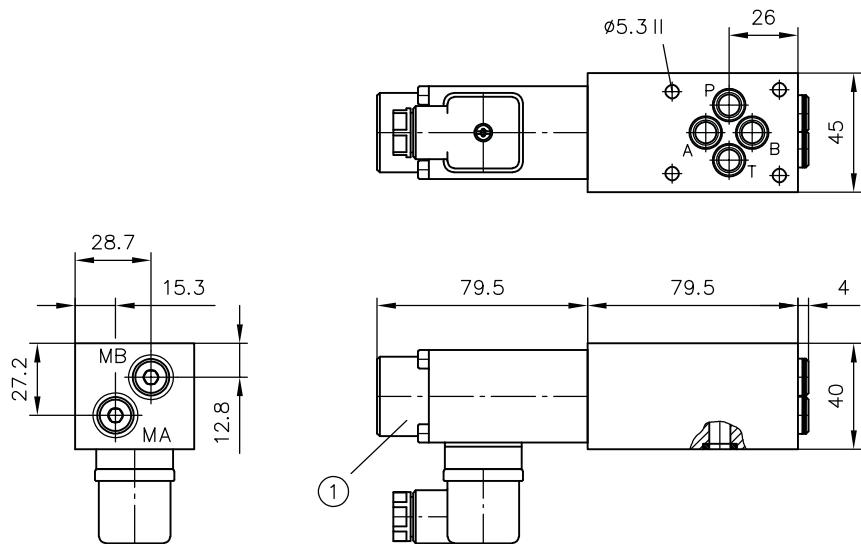
1 Solenoid G..., WG..., X..., for other solenoid versions, see Chapter 4.5, "Intermediate plate with switchable pressure reducing valve at P: NZP 16 LZY"
