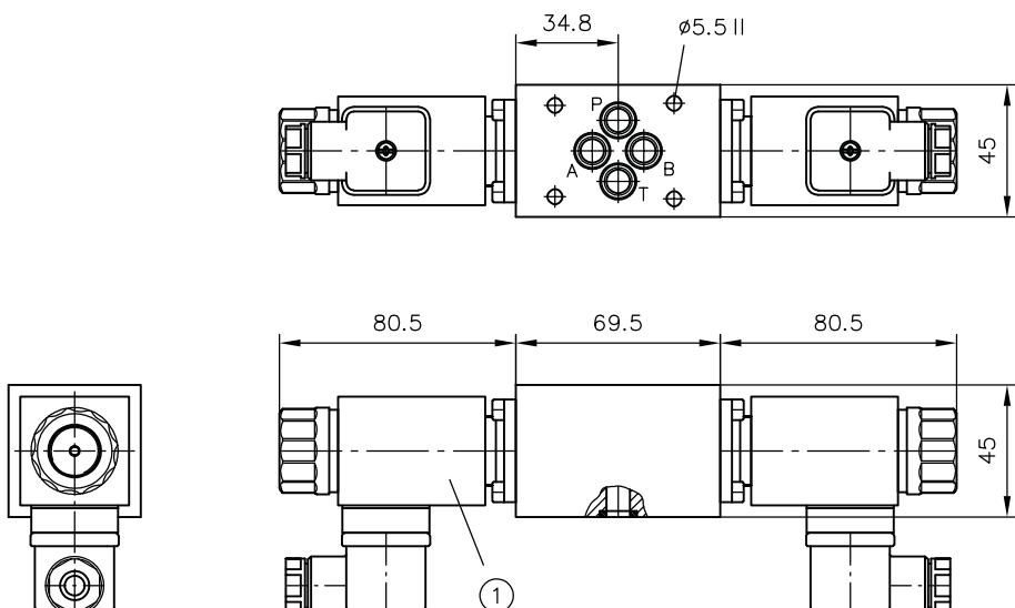
1 Solenoid G.., WG.., X.., for other solenoid versions, see Chapter 4.5, "Intermediate plate with switchable pressure reducing valve at P: NZP 16 LZY"
