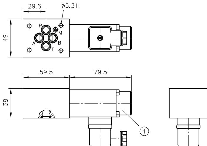
1 Solenoid G.., WG.., X.., for other solenoid versions, see Chapter 4.5, "Intermediate plate with switchable pressure reducing valve at P: NZP 16 LZY"
