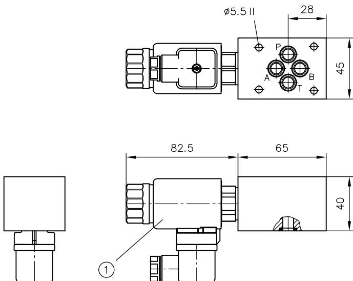
1 Solenoid GM.., WGM.., XM.., for other solenoid versions, see Chapter 4.5, "Intermediate plate with switchable pressure reducing valve at P: NZP 16 LZY"
