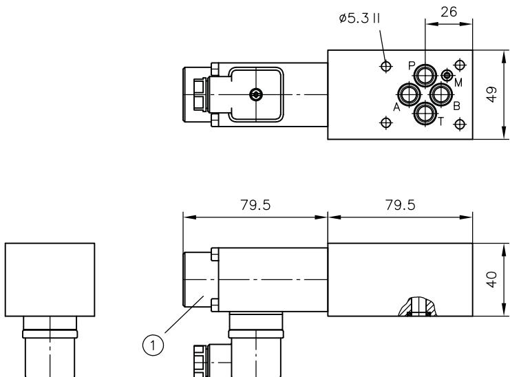
1 Solenoid G.., WG.., X.., for other solenoid versions, see Chapter 4.5, "Intermediate plate with switchable pressure reducing valve at P: NZP 16 LZY"
