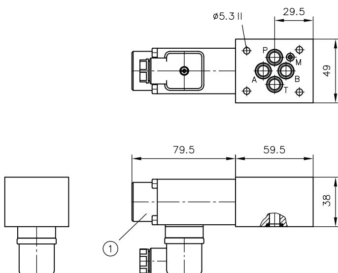
1 Solenoid G..., WG..., X..., for other solenoid versions, see Chapter 4.5, "Intermediate plate with switchable pressure reducing valve at P: NZP 16 LZY"
