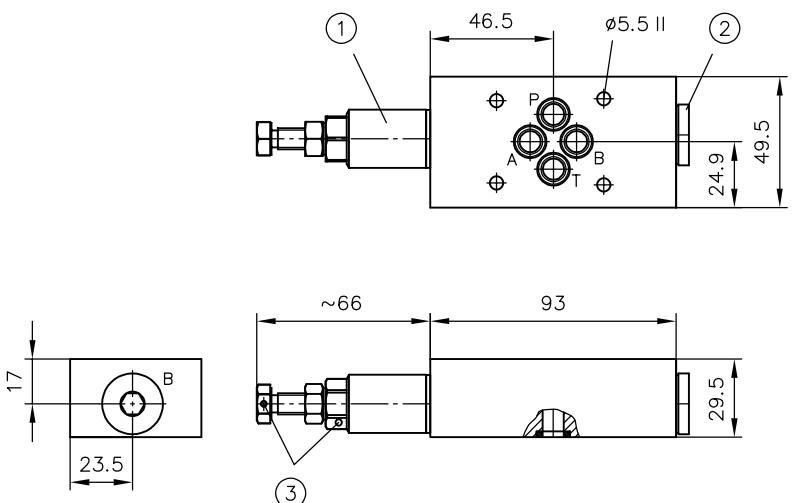
1 Pressure control valve in the A channel
